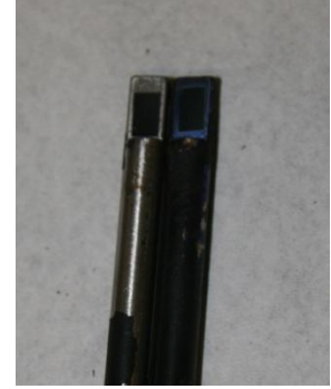
Figure 5.8: Processed Stainless Steel after Electrolysis
