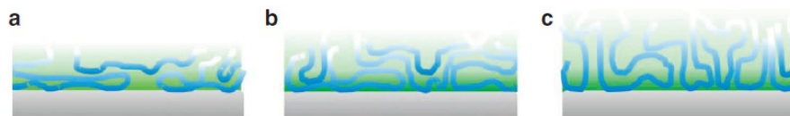
Figure 1-6. The conformations of polymer chains at different annealing time. (a) PS ( M_w = 97K ) annealed for 7.5 mins. (b) PS ( M_w = 97K ) annealed for 2 h. (c) PS ( M_w = 97K ) annealed for 12 h. [20]
