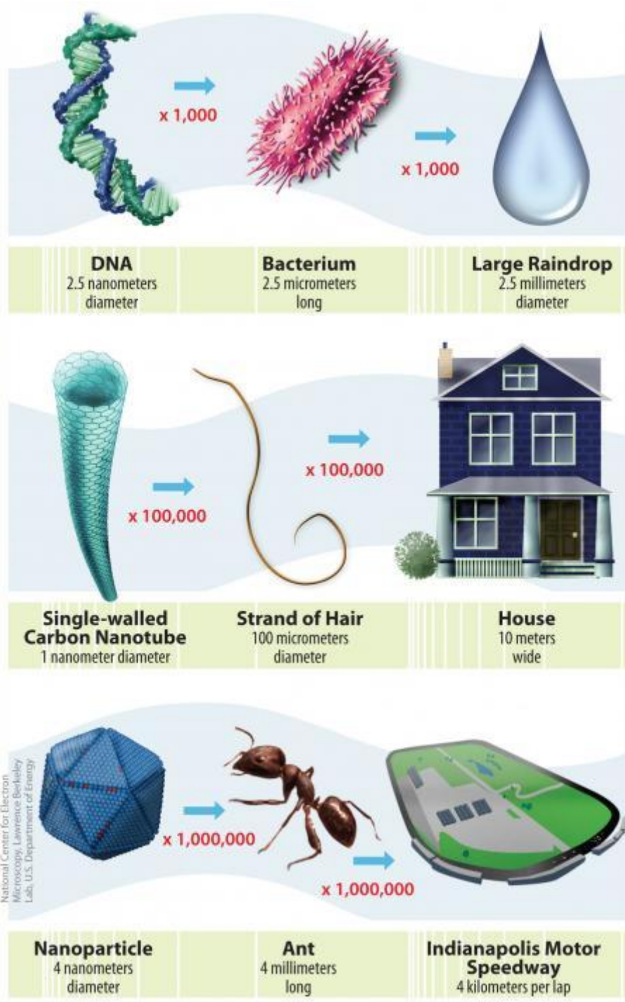
Figure 1.1: Schematic illustration of the scale of nanomaterials vs. macroscale objects. Taken from the National Nanotechnology Initiative ( www.nano.gov )
