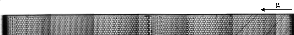
Figure 4-7: -2\ 2\ 0 transmission topograph recorded from edge of the die.
