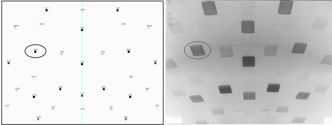
Figure 3-3: (A) A screen shot of LauePt program[48] (HKL)=(-1\ 1\ 0) , (hkl)=(1\ 1\ 0) , \theta_x=5^\circ . Reflection -4 0 -8, indicated in circle (B) An example of reticulographs recorded in reflection geometry and
