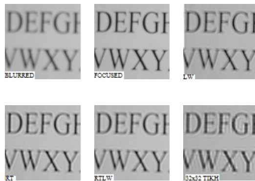
Figure 4.10: Restoration samples from different techniques (at original scale). Order: left – right and top – bottom. Blurred image, focused image, restoration by LW method, RTLW method, RT method and Tikh32.
