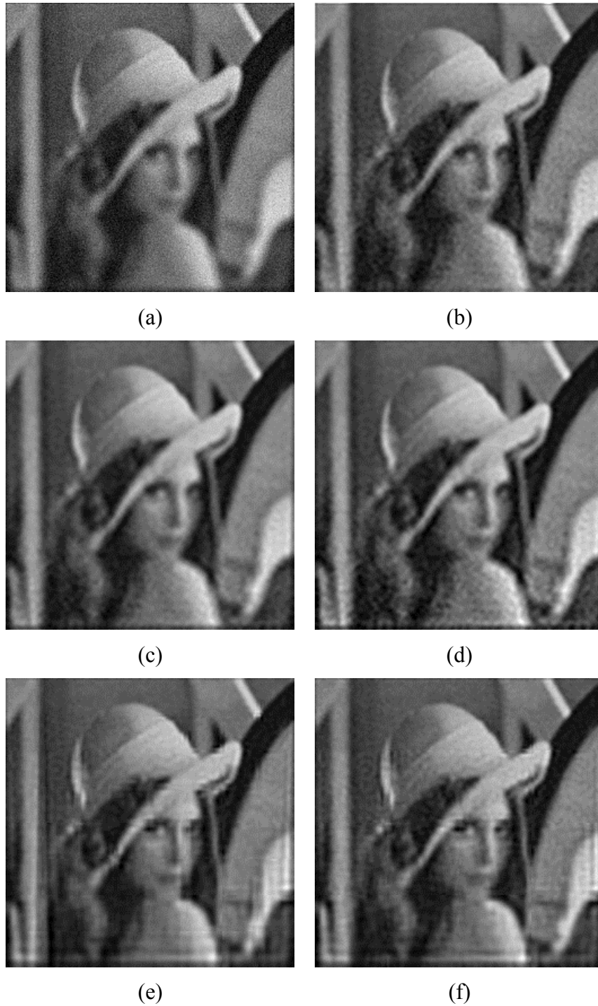
Figure 4.6: Noisy Lena image restoration. (a) Blurred Lena image (with Cylindrical SV-PSFs, radius: 1.5 pixel at the top - 4 pixels at the bottom) at 20dB SNR, Restoration by (b) LW method, (c) RTLW method, (d) RT method, (e) Tikh32 and (f) Tikh64.
