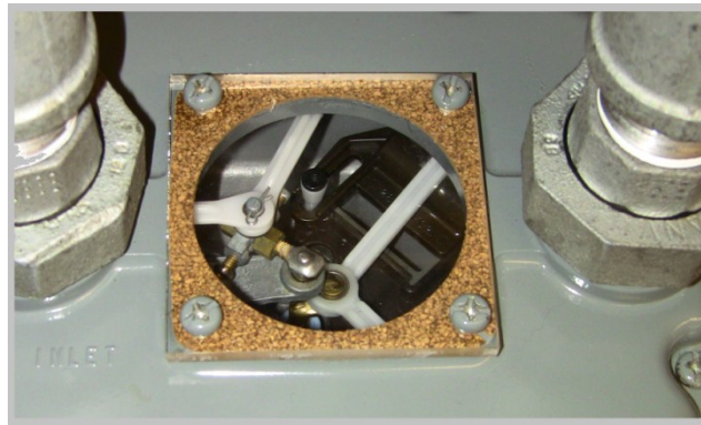
Fig. 2-13 – Acrylic Cover to expose internal meter mechanism
