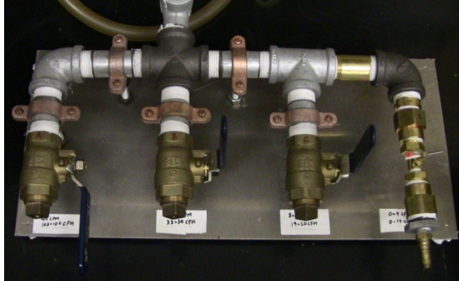
Fig. 2-8 – Valves for simulating constant load and variable load appliances
