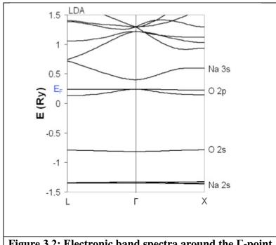
Figure 3.2: Electronic band spectra around the  $\Gamma$ -point
