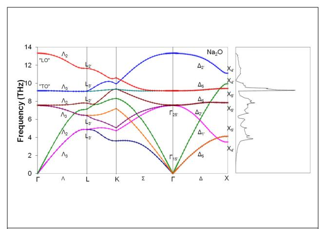
Figure 3.2: Phonon spectra along lines of high symmetry and pDOS from the LDA calculations. Color shown follows the continuous crossing of the modes of different symmetries. Notation along colored lines denotes symmetries as originally proposed by Bouckaert, Smoluchowski and Wigner [25].
