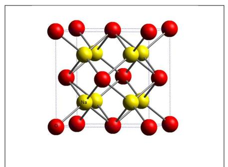
Figure 1.1: FCC crystal structure of Na<sub>2</sub>O.
