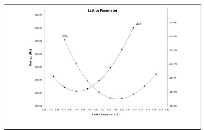
Figure 3.1: Energy plotted as a function of lattice parameter (a). Energies associated with LDA appear on the left y-axis while those associated with GGA are on the right y-axis.
