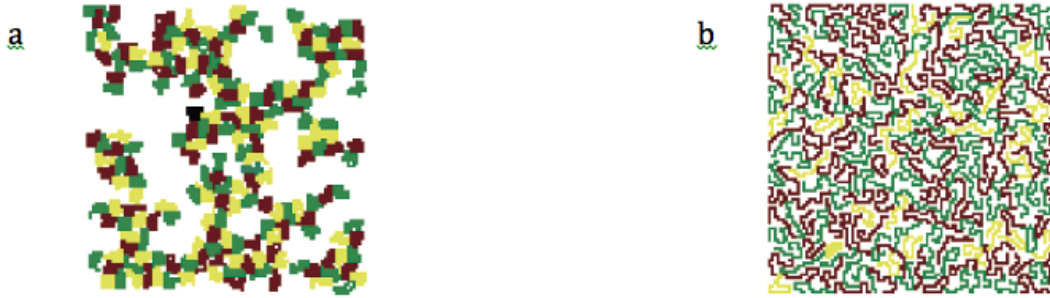
Figure 10. Typical morphologies generated in two dimensional ( 100 \times 100 ) space (a) homophilic chains and (b) heterophilic chains [27].
