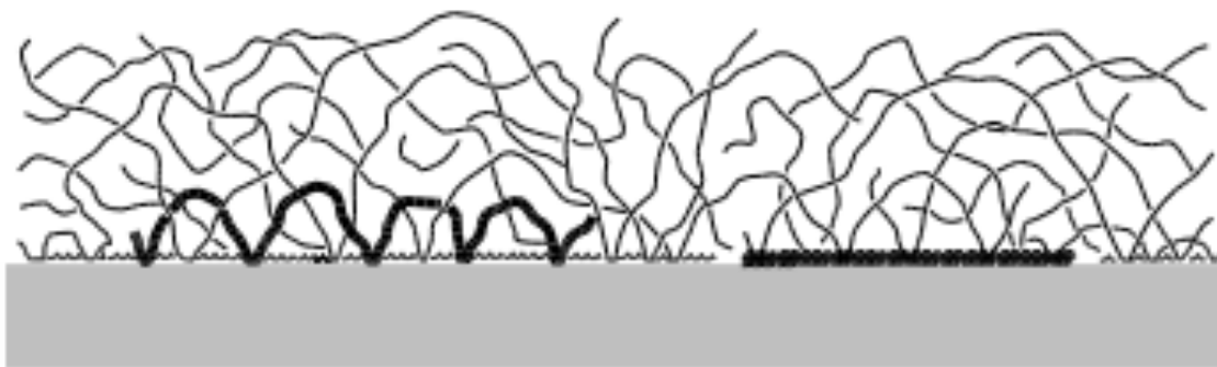
Fig. 3 Sketch of predicted final layer structure resulting from irreversible polymer adsorption. (Ref. 48)
