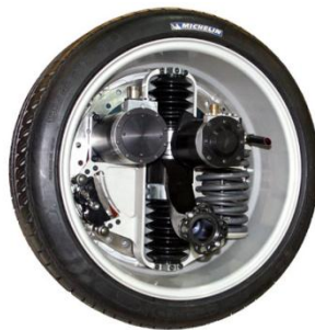
FIGURE 1.6 ACTIVE WHEEL BY MICHELIN
