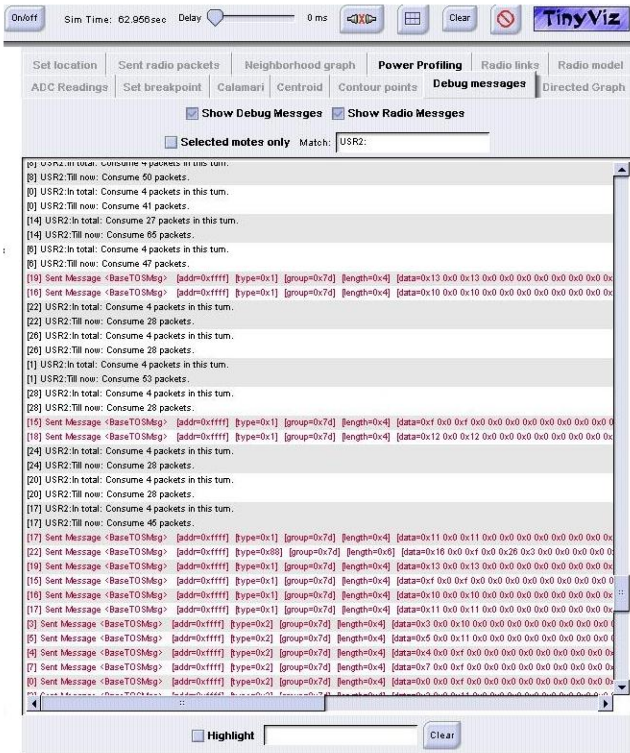
Figure 3.10: Snapshot of the TinyOS LEACH Implementation Running on PowerTOSSIM GUI Displaying the Output Debug Messages
