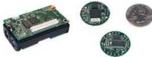
Figure 5.5: Crossbow MICA2 (left) and MICA2DOT (right)
