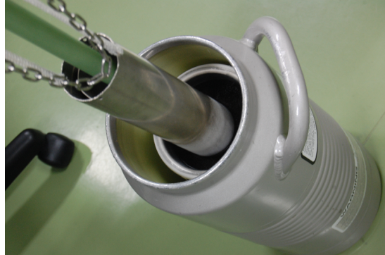
Figure 6.8: Pre-cooling of the 8-bit RSFQ multiplier chip in liquid nitrogen.
