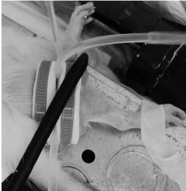
Figure 4.1. Experimental setup. DHS is achieved through a customer design inflatable cuff. The stimulation cuff is connected to an oscillatory actuator-driven syringe, a force-controlled syringe, and a pressure sensor.
