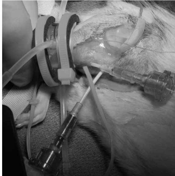
Figure 3.1. Surgical setup. For the ImP measurements, a micro-cardiovascular pressure transducer was inserted into each of the tibial and femoral bone marrow cavities. For bone strain measurements, a single element strain gauge was firmly attached to the flat surface of each of the same tibia and femur over the mid-diaphyseal regions. Simultaneous ImP and bone strain were then measured in the operated tibia and femur under DHS on the tibia.
