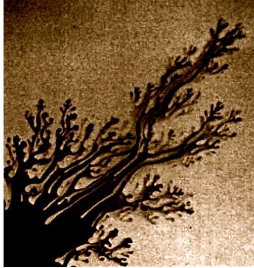
Figure 7: Example of Saffman-Taylor instability in a Hele-Shaw cell.[27]
