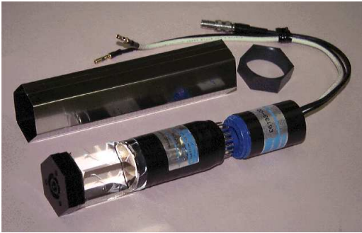
Figure 2.3: A single element of the PHENIX BBC [48].
