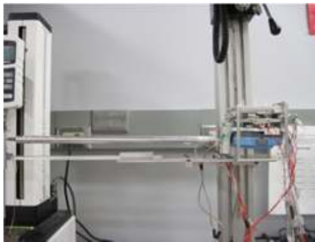
Figure 7.4 Sensor Attachment Installed to Aluminum Frame
