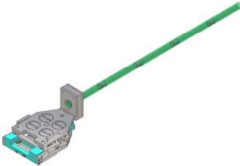
Figure 5.1 Solid Model of Sensor Attachment
