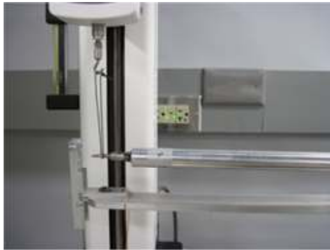
Figure 7.5 Calibrate Tip Force in X-Axis
