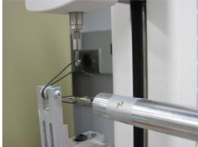
Figure 7.6 Calibrate Tip Force in Y-Axis
