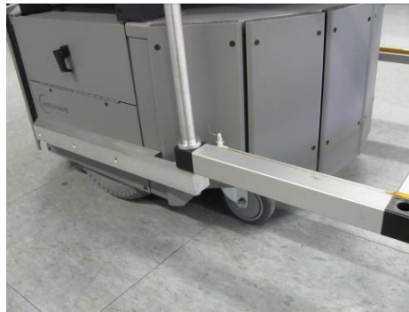
Figure 5.11: Mechanical integration between MMT and robot
