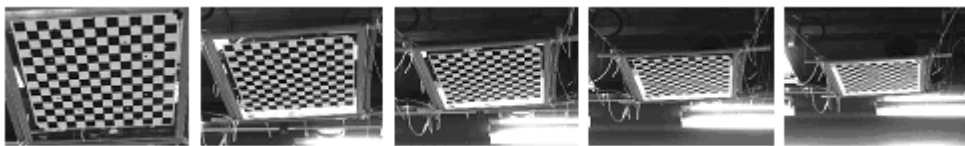
Figure 3.5: Four photos of the pattern are taken from five different distances
