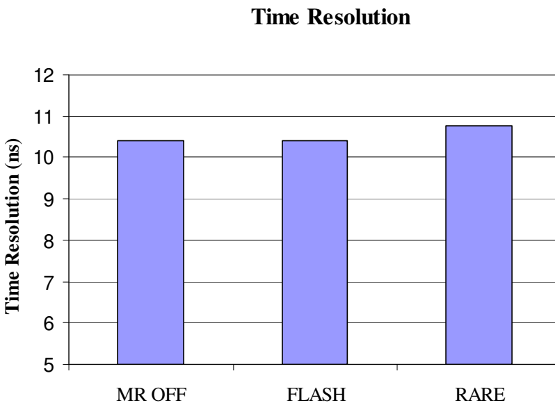
Fig. 5.17. Time resolution comparison for MR OFF, FLASH and RARE sequences using double-layer copper shield.
