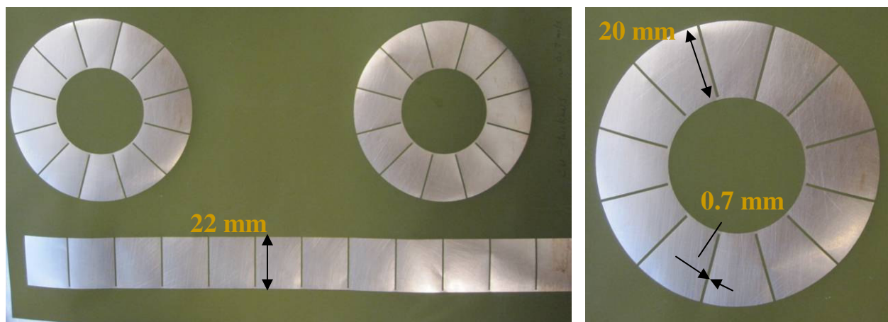
Fig. 6.6. Thin layers of copper with segments etched on a PCB substrate made of kapton.
