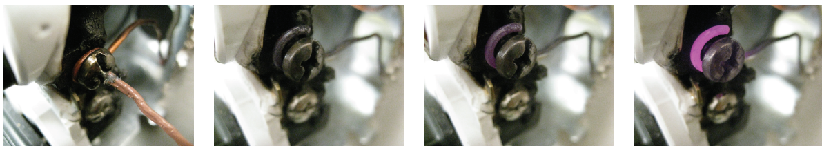
Figure 3.12: Formation and progression of the glowing contact: temperature ranges from 24°C to 280°C
