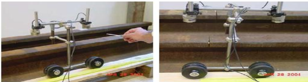
Figure 1.8 Movable sensing system using air coupled EMAT sensors [23]
