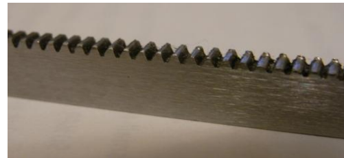
Figure 5.3: Failure of rack in the conventional harvester
