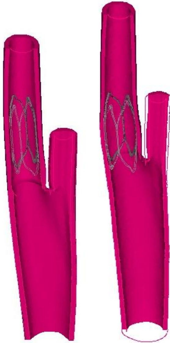
Figure 34. Cross section of carotid artery CA3 with crimped endovascular stent device D6 deployed in ICA.
