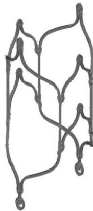
Figure 9. Intra-luminal stent design, in crimped state, employed to distend vascular wall from within the sinus. Dimensions of D5: Height - 17mm, internal diameter - 6.6mm, thickness - 0.2mm.
