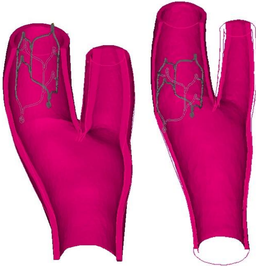
Figure 25. Setup showing stent D5 placed in the sinus of physiologic carotid model CA2 prior to start of simulation (left). Post simulation, image on right, shows carotid wall subjected to 18% axial stretching and stent fully expanded.
