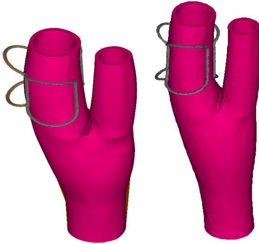
Figure 18. Setup showing device D4 clamped to physiologic carotid model CA2 prior to start of simulation (left). Post simulation, image on right, shows carotid wall subjected to 18% axial stretching and device struts constricting arterial wall radially.
