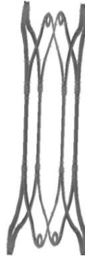
Figure 10. Modified version of stent (D6) in crimped state. Dimensions of D6: Height - 13mm, internal diameter - 2.8mm, thickness - 0.2mm.
