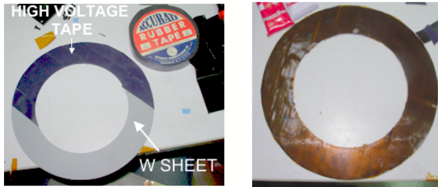
Figure 5.7: A 1mm thick W sheet for background shielding, covered with high voltage rubber tape and Kapton tape(right)
