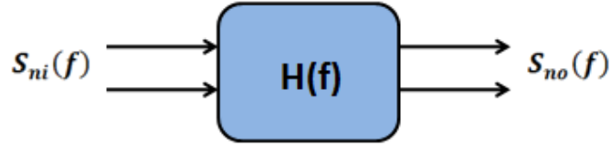
Figure 2.3 Linear Time-Invariant System with Transfer Function H(f)
