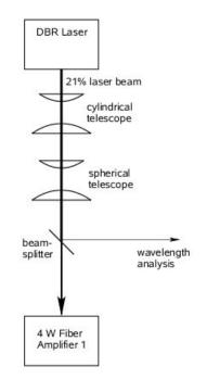
Figure 4.12 The origin of the Optical Pumping beam. The 21% laser beam is brought to a useful shape by a cylindrical and a spherical telescope. After that it is split, where one part is used for wavelength analysis and the other part is sent to a 4 W YDFA to provide the optical pumping beam and the SAS feedback.
