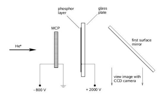
Figure 3.5 Picture of the MCP/PS detector system for the detection of the original and the deflected He\*-beam. The mirror that is mounted in a 45 angle to the beamline is used to reflect the image through the side window of the vacuum chamber, so that it can be viewed with a CCD camera without interfering with atomic lithography at the end of the beam.
