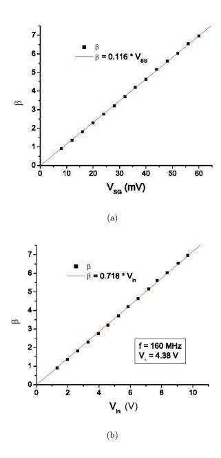
Figure 5.2 (a) The calibration curve of the phase modulation index  $\beta$  vs. the signal generator voltage  $V_{\rm SG}$ . (b) The calibration curve of  $\beta$  vs. the input power of the phase modulator  $V_{\rm in}$ .  $V_{\pi}$  was measured to be 4.38 V for the modulation frequency  $\omega_{\rm pm} = 160 \text{MHz}$  [13].
