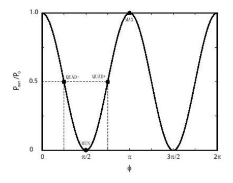
Figure 4.6 Power (vertical axis) against phase shift (horizontal axis) on one arm of the Mach-Zehnder amplitude modulator. Since the phase shift on the other arm has the same magnitude but opposite sign, the total phase shift has to be doubled. Possible operating points are also shown in the plot. In this experiment, the minimum was used as operating point [13].
