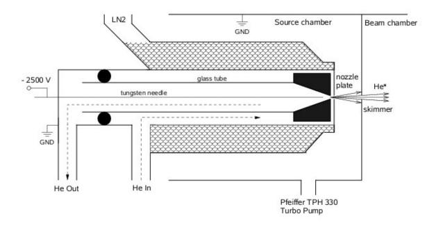
Figure 3.2 Cross section of the DC discharge source for the production of metastable Helium. Note that the ceramic spacer on the tungsten needle is not shown.
