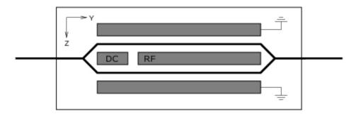
Figure 4.5 Schematic layout of an amplitude modulator. The principle axes of the crystal are shown in the upper left corner of the graph.
