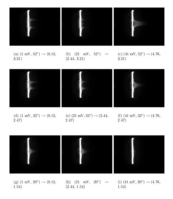
Figure 6.8 A fraction of the images that have been taken for the Force-Mapping. The Parameters are indicated below each image:  $(V_{SG}, \theta_{\frac{\lambda}{2}}) \rightarrow (\frac{\delta_0}{\omega_m}, \frac{\Omega_0}{\omega_m})$ . Again, the magnetic field has a value of  $B \sim (7 \pm 0.5) \times 10^{-4} \text{ T}$ .
