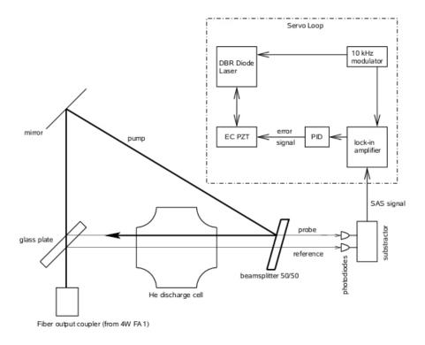
Figure 4.2 The Saturated Absorption Spectroscopy is used to lock the laser frequency reliably on the transition frequency of  $2^3S_1 \rightarrow 2^3P_2$ . In the lower part of the picture it is shown how the SAS-Signal is derived from the part of the Optical Pumping beam that was split behind the 4W FA. The Servo Loop in the dashed box shows how the SAS signal is used to produce electronic feedback to the laser for frequency stabilization.
