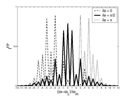
Figure 5.5 Numerical calculation of the FP-spectra of the light pulses in figure 5.4(d) using equation 5.28. The settings are the same as in figure 5.4[13].
