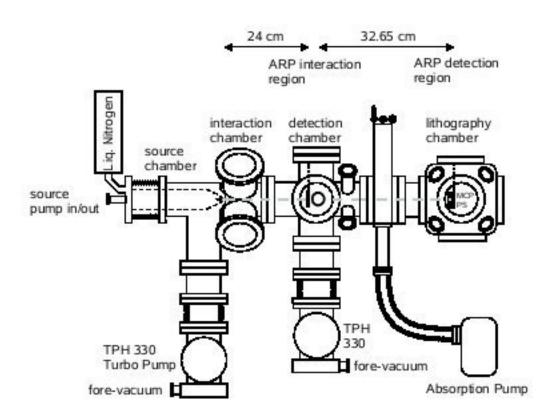
Figure 3.4 Schematic of the vacuum system viewed from the side. The names of the chambers correspond to the lithography experiment.
