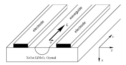
Figure 4.3 The schematic of a X-cut LiNbO<sub>3</sub> modulator. The light propagates in the Y-direction  $(\vec{k})$  and the two electrodes, that are also along the Y-axis produce the electric field along the Z-axis for modulation.  $\vec{e}$  represents the polarization axis in the crystal.
