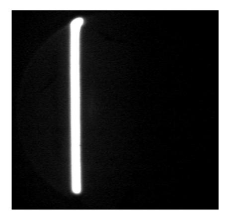
Figure 6.2 Undeflected atomic beam. The view is towards the source and the slit that geometrically defines the atomic beam is imaged on the screen.
