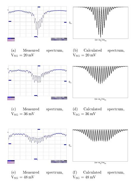
Figure 5.6 Measured (left) and calculated (right) FP spectra of the modulated light after the 4W YDFA. The calculations have been done with equation 5.28. The DC bias voltage on the amplitude modulator is nearly zero [13].
