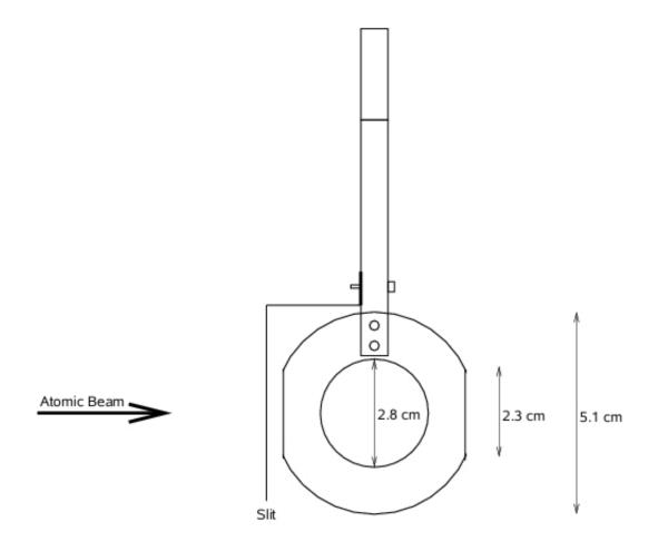
Figure 3.7 Sideview of the Helmholtz-coils including mount and slit for the atomic beam (perspective of the laser beams). All measures are given in cm.
