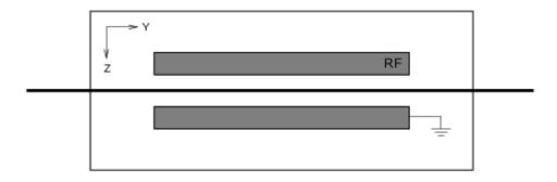
Figure 4.4 Schematic layout of a phase modulator. The principle axes of the crystal are shown in the upper left corner of the graph.
