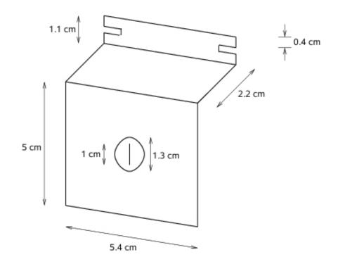
Figure 3.8 Schematic of the slit for the atomic beam. A thin metal foil is glued on an aluminum piece and a slit is cut into the foil. The length of the slit is 1 cm and its width is 250  $\mu$ m.
