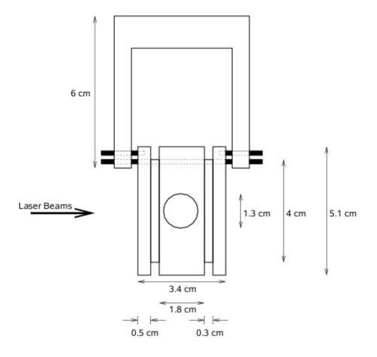
Figure 3.6 Frontview of the Helmholtz-coils with mount (perspective of the atomic beam). The hole in the middle is for the atomic beam and the laser beams (ARP and OP) are perpendicular to it. The slit for the atomic beam is not shown here. Sizes are given in cm.
