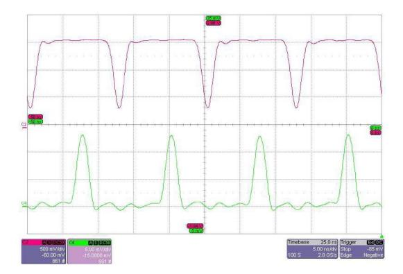
Figure 4.7 Image of the periodic optical pulse delivered by the NIR-MX-LN03 AM (lower image) and the complement of the RF drive signal (upper image). The frequency of both signals is 80 MHz and the pulse width is about 3.5 ns. Note, that the optical signal shows some ringing at the base which might be induced by the after-pulse tail of the electric signal together with some RF reflection.
