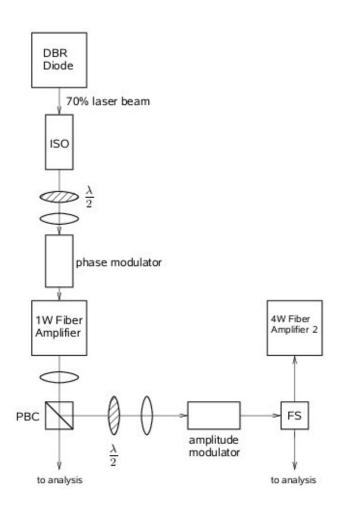
Figure 4.10 After the 70% beam of the DBR laser went through an isolator it is brought into the phase modulator. The output of the phase modulator is preamplified by a 1 W YDFA and then lead into the amplitude modulator. The result is a chirped pulse and is sent through a fiber splitter to the 4 W YDFA in order to rise the power to a useful level for the experiment. The light that is split after the fiber splitter and the 1 W and the 4 W YDFA is used for spectrum analysis.
