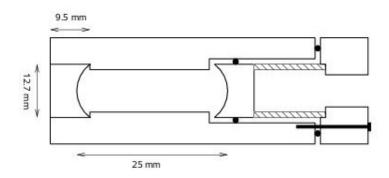
Figure 4.9 Schematic of the Fabry-Perot spectrometer. The length of the cavity is 25 mm, the mirror diameter is 12.7 mm, their focal length is also 25 mm and the thickness 9.5 mm.
