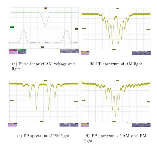
Figure 5.4 The Fabry Perot spectra of the modulated light pulses. Settings:  $V_{SG} = 20 \text{ mV}$  (phase modulator),  $-\frac{V_a}{8} \text{ DC}$  bias of the AM voltage, where  $V_a$  is the voltage on the amplitude modulator [13].
