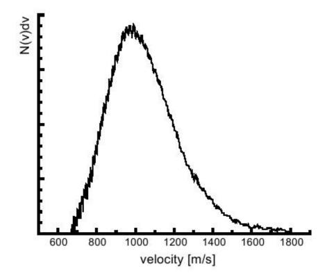
Figure 3.3 Longitudinal velocity distribution of metastable He-atoms with a discharge current of 6 mA as measured in [41].
