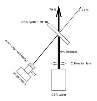
Figure 4.1 The light that leaves a diode laser is first collimated by a collimation lens and then split by a 70/30 beamsplitter. The 70% of the beam are sent to the modulators and are finally used for the experiment. The 30% light is retroreflected by a high reflectivity mirror (>99%) and split again at the beam splitter, where 9% of the light is used as an optical feedback for the laser and the remaining 21% is used for optical pumping, wavelength analysis and SAS (after amplification).
