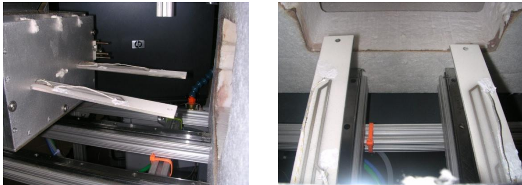
Figure 2-5: Setup to measure the Seebeck coefficient for the sprayed TSTC.
