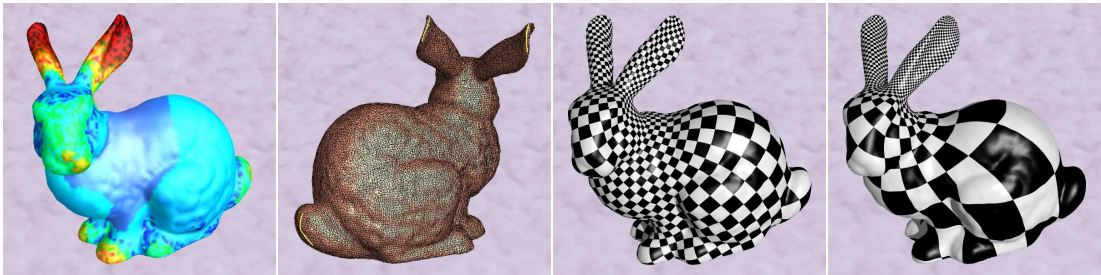
Figure 9: Bunny Model With Topological Optimization. (a).Conformal Factor is color encoded into bunny (b). Topological Optimization: three slices in bunny (c). Most Uniform Global Conformal Parametrization, energy: 0.37e-4 (d). Least Uniform Global Conformal Parametrization, energy: 2.1e-4
