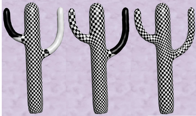
Figure 8: Cactus Model. (a).Most uniform parametrization with cactus model (b). Most uniform parametrization after one slice on the top of the left branch (c). Most uniform parametrization after another slice on the top of the right branch.
