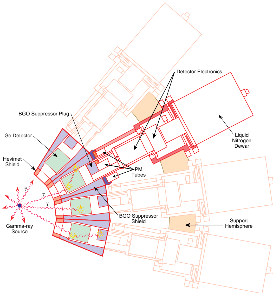
Figure 4.2: A schematic diagram of Gammasphere HPGe detectors. It consists of a HPGe crystal, BGO anti-Compton elements, photomultipliers for the BGO elements, Hevimet collimators, detector electronics, and a liquid nitrogen dewar, which stores liquid nitrogen for cooling the HPGe crystal. (Figure from Ref. [50])
