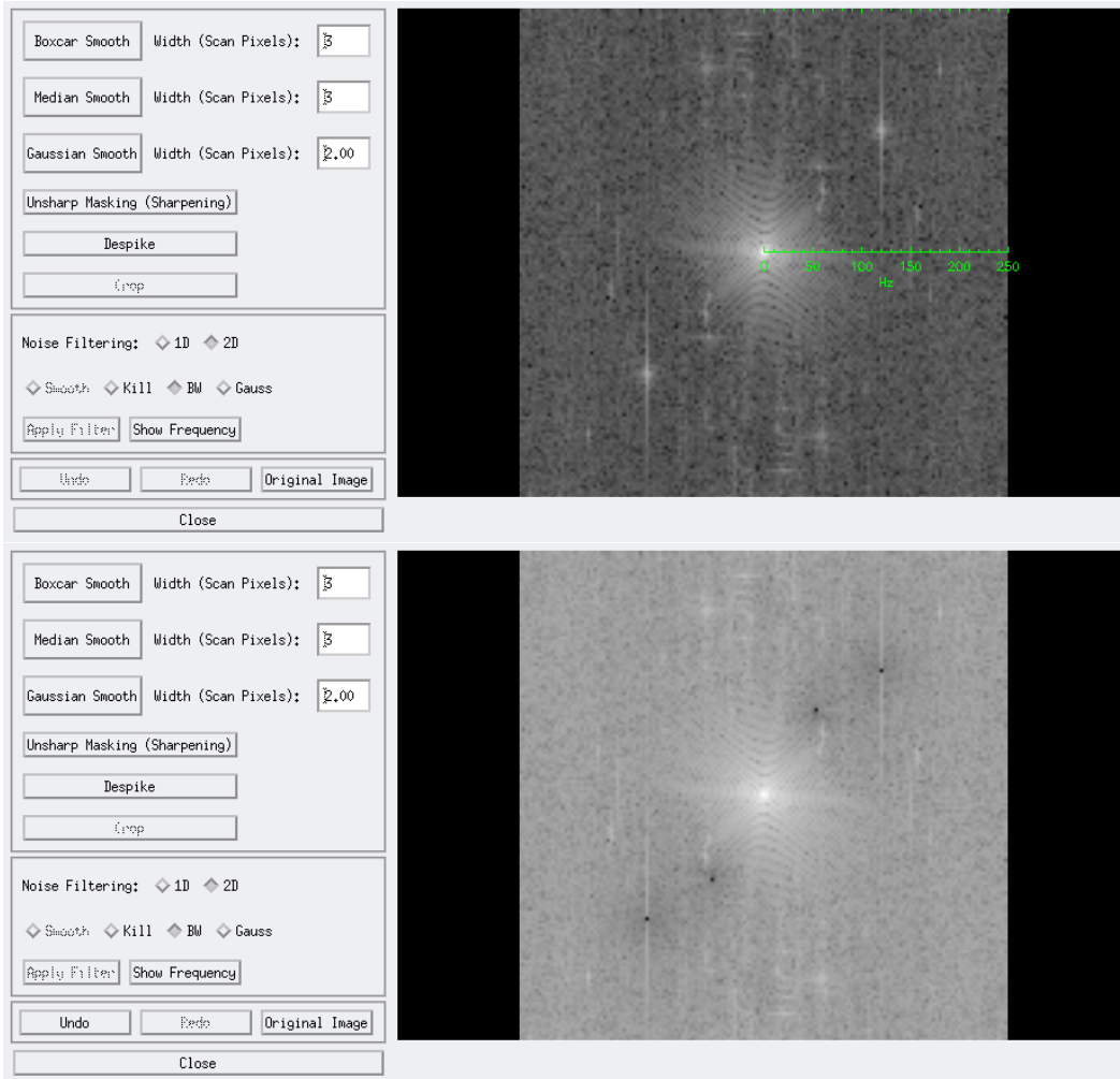
Figure 2.16: Fourier transform for noise filtering. The upper image shows the 2D Fourier transform of the noisy image. Overlaid in green is an axis of corresponding temporal frequencies. The lower image shows the Fourier transform after applying a Butterworth filter at two different points.
