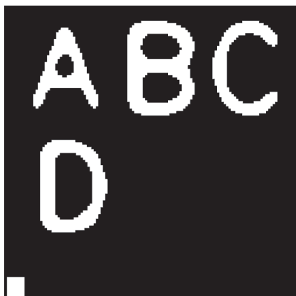
Figure 3.1: The black area in the first test specimen was assigned the transmission spectrum of 110 nm of collagen, 60 nm tyrosine and 30 nm leucine. Letter A was assigned the transmission spectra of 100 nm of collagen and 100 nm of leucine, B 100 nm collagen and 100 nm tyrosine, C 20 nm of collagen and 180 nm of leucine, D 20 nm of collagen and 180 nm of tyrosine. The square at lower left was assigned to be nonabsorbing so as to provide an I_0 flux normalization region.
