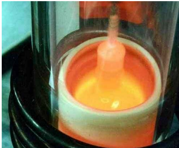
Figure 4 A growing single crystal by the Cz method (originated from ICMCB-CNRS)
