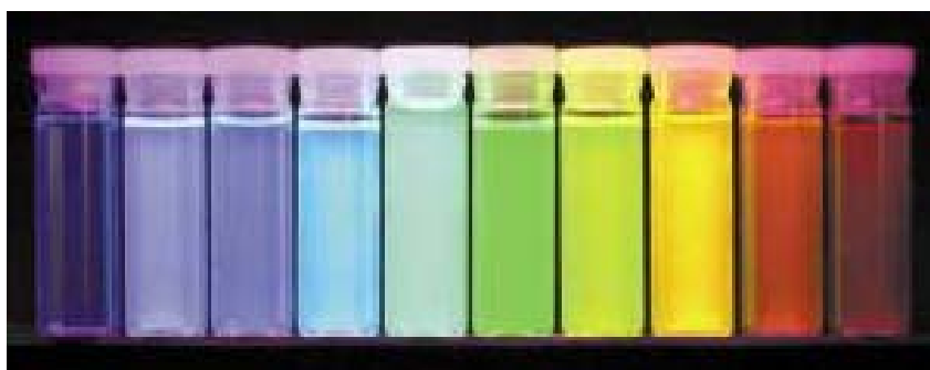
Figure 4-6. Ten distinguishable emission colors of CdSe/ZnS QDs. 32 (Figure is adapted from Ref. 32)
