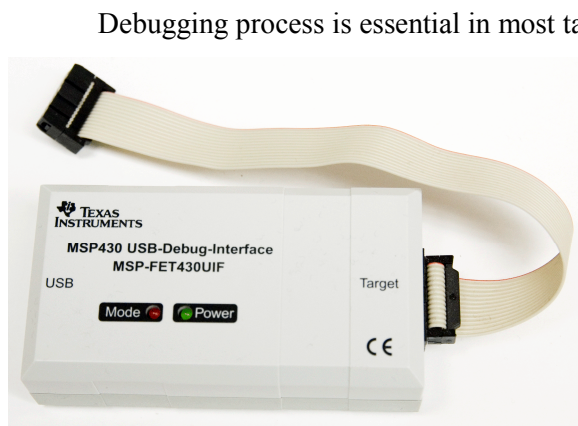
Fig. 7-1. The MSP-FET430UIF Debugger
