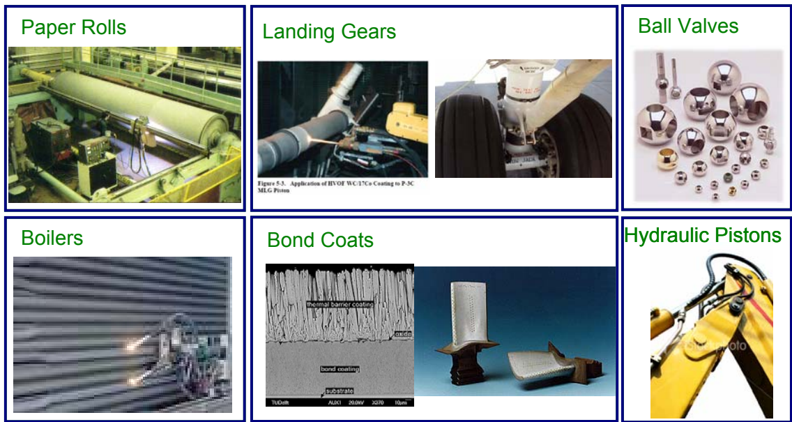
Figure 1-6. Traditional applications of HVOF coatings for several engineering components
