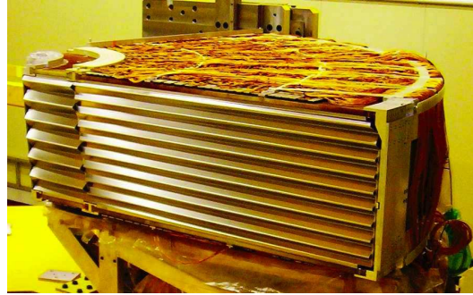
Figure 3.6: Module of the EMB calorimeter shown during assembly. Eight such wedge-shaped modules combine to form a wheel.
