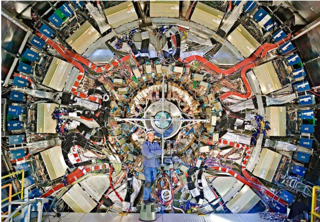
Figure 5.6: This picture of the services in the transition region (SIDE A) highlights the complexity and diversity of the materials to be described. Note the intricacy of the routing of services.
