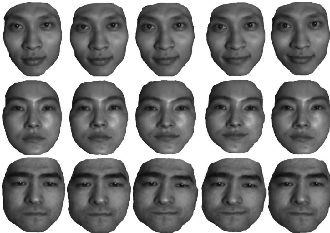
Figure 34: Exaggerated expression transfer. Source face model with exaggerated expressions are shown in the first row. Transferred expressions on two target faces are showed in the second and third row, respectively. The target faces have different shapes and textures but the expressions are proportionally scaled to fit each model well.
