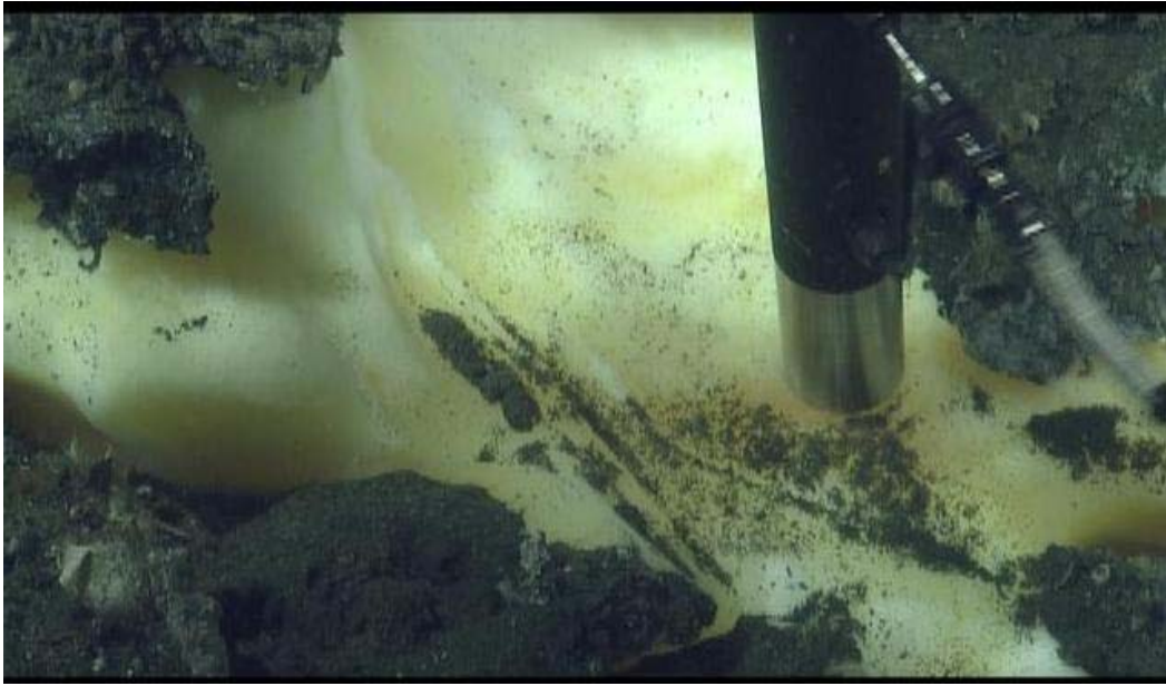
Figure 4.7 Massive mudline hydrates, Barkley Canyon, British Columbia, Canada (Monterey Bar Aquarium Research Institute, 2006)
