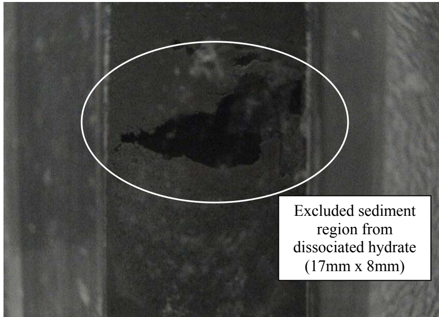
Figure 4.5 Geometry of the host sediment subsequent to complete dissociation of methane hydrate formed in Figure 4.4.
