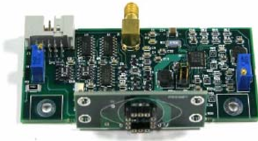
Figure A.7 Photo of fabricated PCB. 32-channel photon detection module is based on this PCB.
