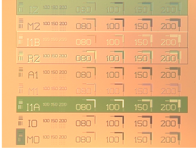
Figure 3.6: A micrograph of photolithography monitoring structure containing an array of circular features, lines and spaces and CD bars placed on all layers, providing the visual clue and control mechanism.
