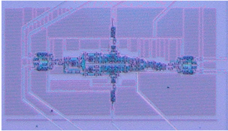
Figure 5.7: Micrograph of streaming I/Q mixer implemented in 4.5 \text{ kA/cm}^2 .
