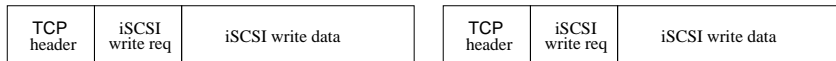
Figure 5.3: Skew in location of common data because of dissimilarity in TCP stream contents. Connection 1 write data gets displaced because of interspersed READ requests.
