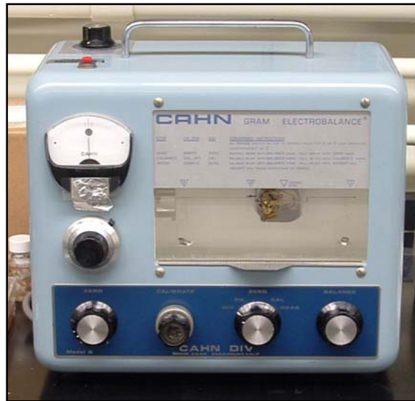
Figure 4.4 – Cahn microbalance used to measure ossicular mass.
