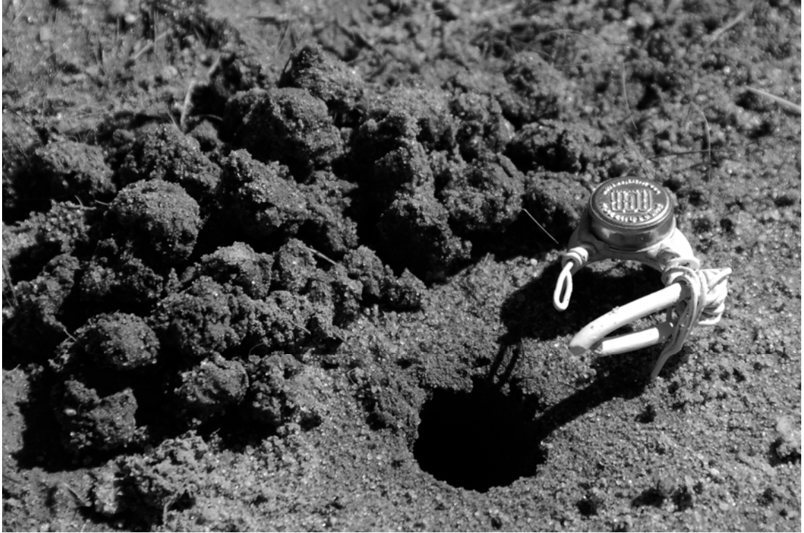
Figure 1. A fiddler crab thermal mimic next to a burrow in the high intertidal sand flat breeding area of Uca pugilator .
