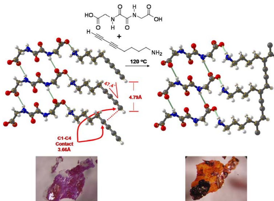
Figure 3.1 The topochemical polymerization of salt (66dH) 2 OG . The partially polymerized monomer salt crystals turned from blue to yellow polymer crystals smoothly.
