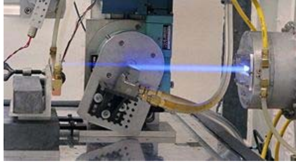
Figure 1.2: x-rays emerging from a synchrotron beam port excite nitrogen in the air resulting luminescing blue – Image obtained from www.nsls.bnl.gov .
