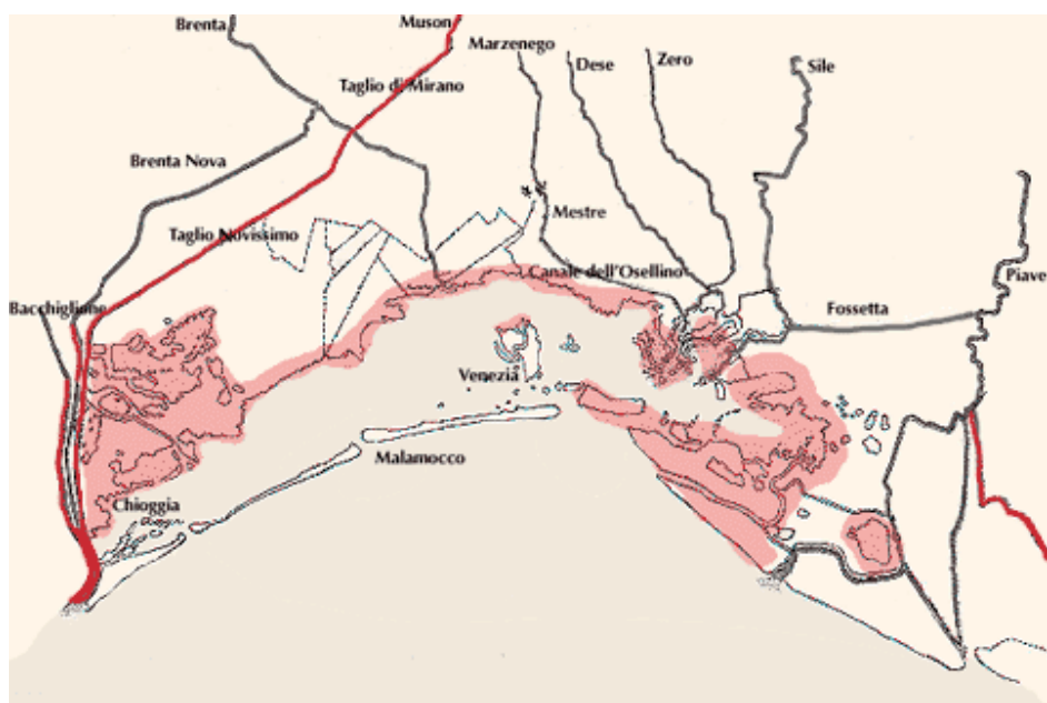
1600: Emplacement of sand and other sediment around the lagoon to stabilize its borders
