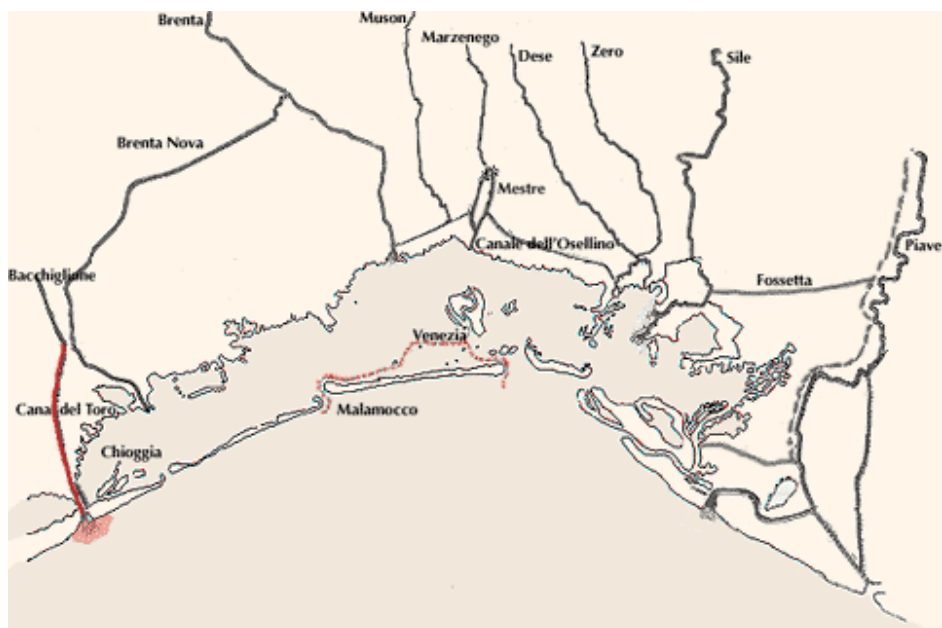
1550: Diversion of the Brenta River out of the lagoon. Dredging of a deep navigation channel from the Malamocco inlet to the city.
