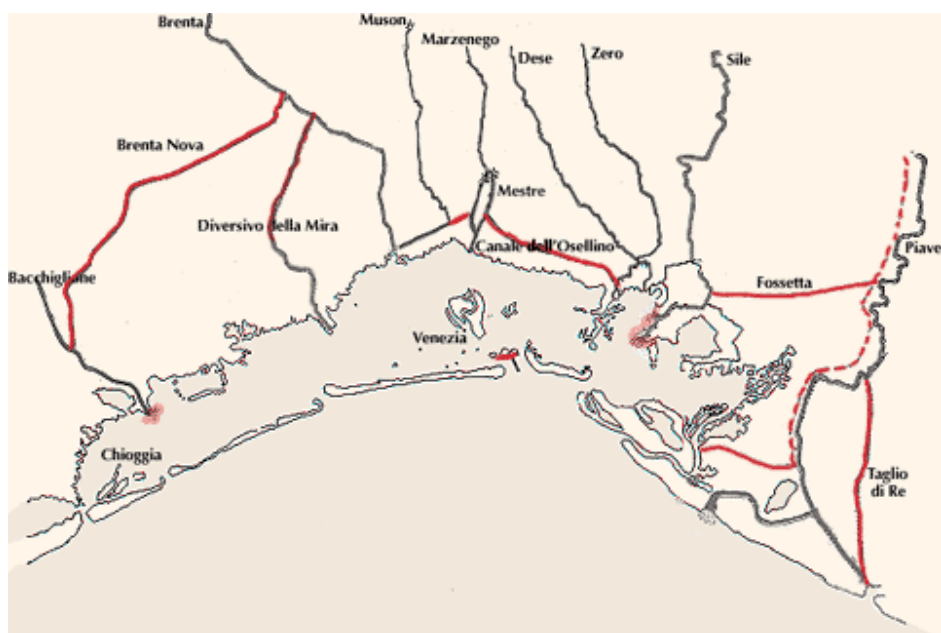
1500: Diversion of Brenta River further south and the Piave River out of the lagoon. Fortification of the Lido inlet.
