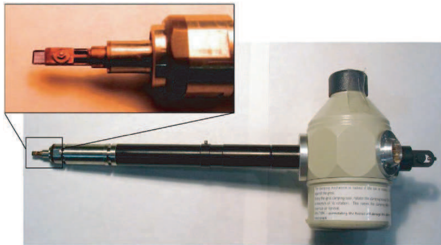
Figure 3.6: A picture of the Gatan 630 Cryo-holder with a enlarged view of its tip with grid in.
