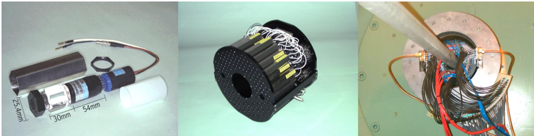
Figure 2.4: The Beam-Beam Counters. Left: A single element consisting of a PMT and a quartz radiator. Middle: One of the two assembled BBC detector arrays. Right: BBC array cabled and installed around the beam pipe on the face of the central magnet.
