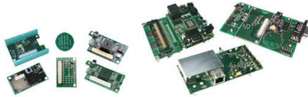
Figure 2.3: Sensor/Data Acquisition Board (left) and MIB Board (right)
