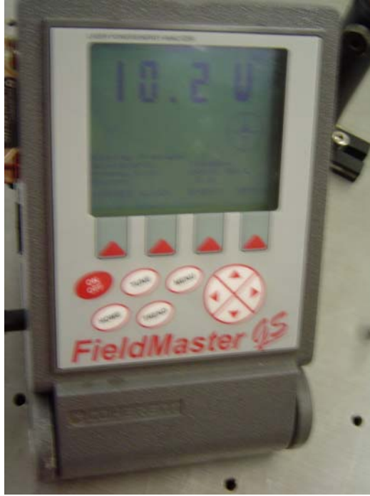
Figure 16: Powermeter to measure the experimental probe beam reflectivity
