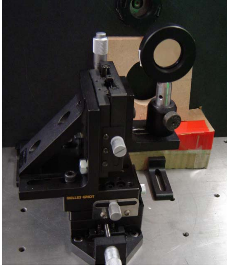
Figure 29: Specially-built translation stage with 100mm-focal lens
