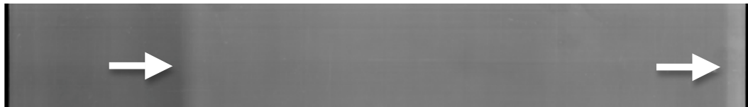
Figure 31 – Banding artifact seen on Vidar DosimetryPro 16 visible on the top and bottom of the film. Film is shown rotated 90° clockwise with contrast enhancement to show artifact.
