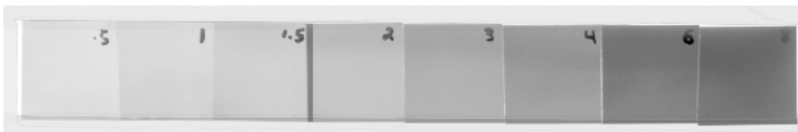
Figure 26 – Example of scan obtained from the Vidar DosimetryPro 16 for determination of the digitizer sensitivity.
