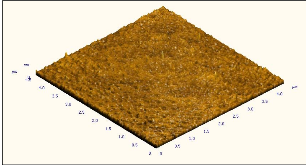
Figure 3.5: Three dimensional topography of the bulk silica substrate obtained with AFM. The bulk silica substrate is an analog of an oxide layer and this sample has the RMS roughness of about 0.35 nm (Scan size: 5 μm by 5 μm).
