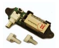
Fig. 21. Small power supply for modulated LED light source.
