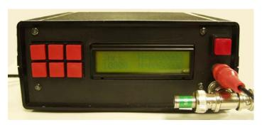
Fig. 56. Fully adjustable control signal sequence generator with indication of control signal parameters and counting results.
