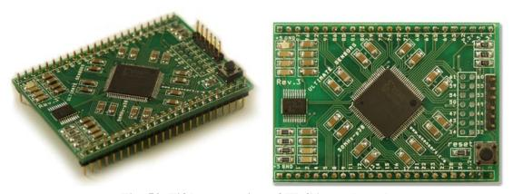
Fig. 53. Fifth generation of FPGA coreboard.
