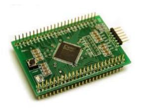
Fig. 52. Fourth generation of the FPGA coreboard.
