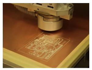
Fig. 50. LPKF ProtoMat C30S. Making top layer of FPGA core unit.
