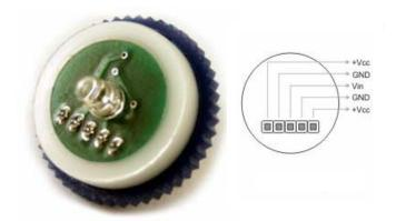
Fig. 20. Fast modulated LED light source and its pin description.
